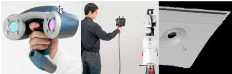
Figure 4. The Creaform MaxScan (left) requires targets and the Leica system (center) monitors and reports position via laser tracker. The scan data (right) is the result of these handheld tools.
