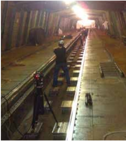
Laser Trackers are used to measure Aircraft Carrier Catapult Rails.
